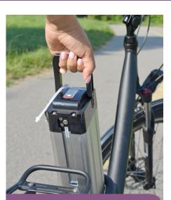
When lithium-ion batteries fail they can get very hot very fast. They can burst violently, hiss and release toxic, flammable and explosive gases. This can cause a very intense fire that is difficult to put out.
