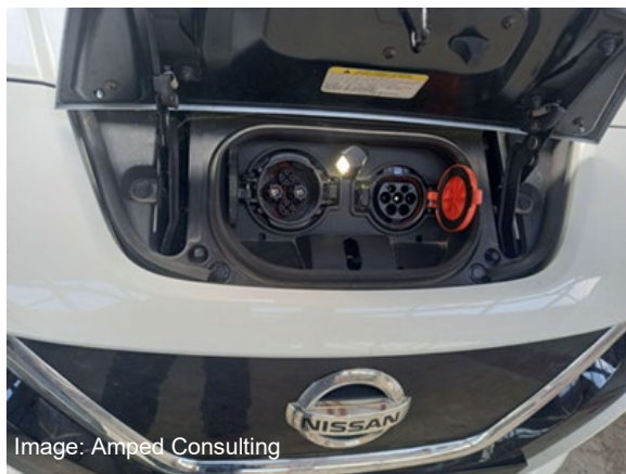
CHAdeMO (left) and Type 2 port on a Nissan Leaf
